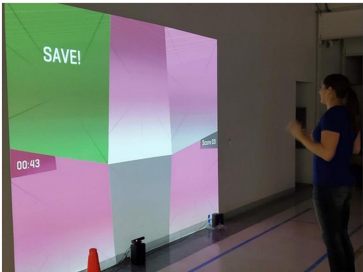
Figure 16: User testing an early prototype of the goalball game with Olympic and Paralympic athletes. Here, an approximation of the hardware setup was created with speakers mounted above the projection and below. The main thing we learned from this session was how detailed calls to action needed to be to allow visitors to participate intuitively in a motion-led game. Credit: CRÉO Exhibits.
