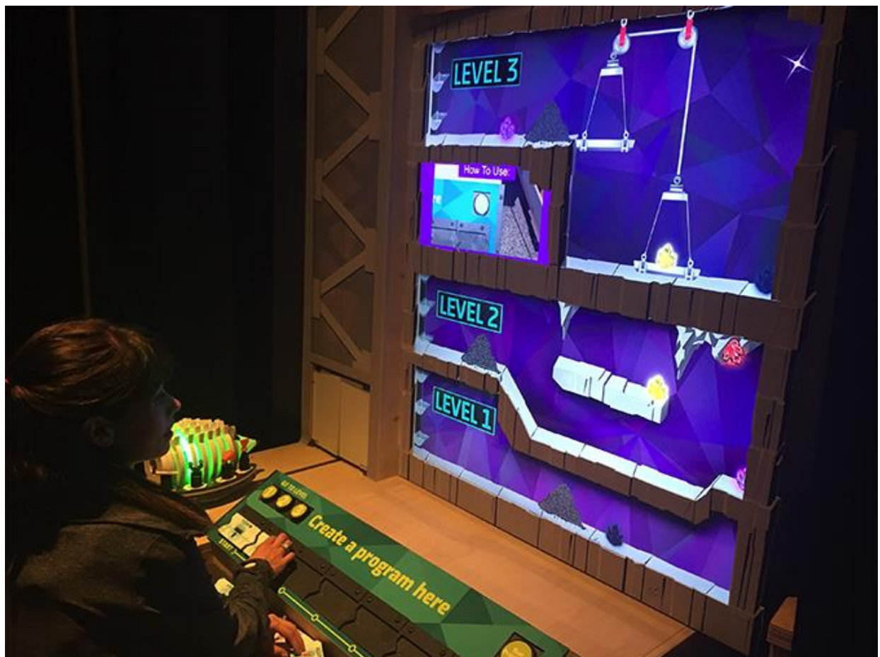
Figure 11: In the “Robots” prototype, visitors can use physical blocks to program a physical robot before sending it to collect gems in a virtual world. Photograph by Bill Jackson. Courtesy of the Museum of Science, Boston.
